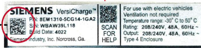
The carrier scans the Data Matrix barcode on the Siemens EVSE using the MDD TR
