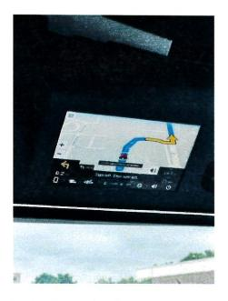
Turn by turn copilot mapping displays in landscape mode on the vehicle monitor. The turn by turn direction speech comes from the vehicle speakers. The level of the volume can be controlled by the volume icon on the bottom of the monitor display while the vehicle is in Park, the controls cannot be adjusted while driving or if the vehicle is in Drive/Reverse for safety reasons.
