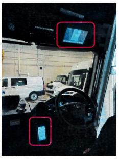
Once the device is cradled in the vehicle cradle, the MDD screen will be displayed on the vehicle monitor, while the vehicle is in park.
