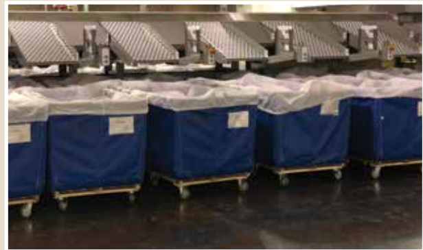
The hampers have a bungee insert that rises as the load decreases so employees do not have to bend over into a hamper to retrieve mail from the bottom. The center will have Small Parcel Bundle Sorters (SPBS) that will enhance sorting parcels and bundles.
