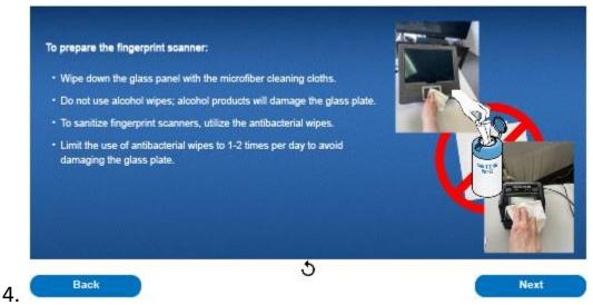
To prepare the fingerprint scanner, first wipe down the glass panel with the microfiber cleaning cloths that are included in the fingerprint workstation kits. Do not use alcohol wipes to clean the fingerprint scanners as alcohol products will damage the glass plate. To sanitize fingerprint scanners, utilize the antibacterial wipes that are included in the fingerprint workstation kits. Limit the use of antibacterial wipes to 1-2 times per day to avoid damaging the glass plate.
