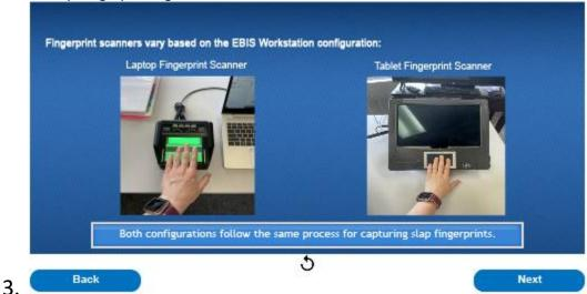
Before we begin, it is important to note fingerprinting scanners vary based on the configuration of the EBIS workstation. EBIS laptop workstations have an ancillary fingerprint scanner connected to the laptop. EBIS tablet workstations have a fingerprinting scanner integrated into the tablet while the physical component of the fingerprint scanner may vary between a laptop and a tablet workstation, both configurations follow the same process for capturing slap fingerprints.
