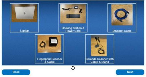
The EBIS laptop workstation consists of the following components: a laptop, docking station and power cord, ethernet cable, fingerprint scanner and connection cable, and a barcode scanner with cable and stand. Please note, that while a laptop power cord will be included in the kit, it will not be used as the laptop will be charged via the docking station.
