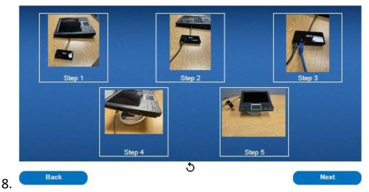
To setup the EBIS tablet workstation, first connect the dongle to the tablet. Second, connect the tablet power cord to the dongle. Third, connect the ethernet cable to the dongle. Fourth, place the tablet on the stand. The fifth and final step is to connect the remaining end of the ethernet cable to a working network port and connect the power cord to a working outlet. Note, the EBIS workstation must be hardwired to the USPS network and cannot be on WIFI.
