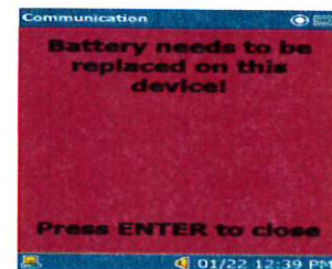
Battery in bad condition and shall be replaced. (Cycle count >425)
