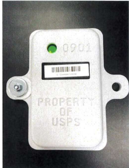
GPS device in protective clamshell (case) showing battery indicator light and barcode
