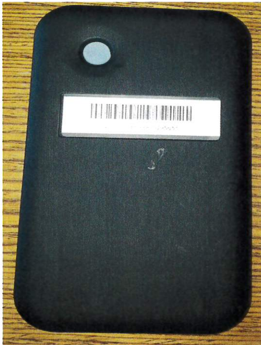
GPS device without case showing battery indicator light and barcode
