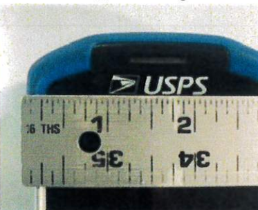
MDD-TR 1" from left edge to lead edge of Eagle emblem. 2" from left edge to lead edge of 2 nd "S"
